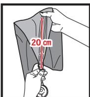
When injecting gas with the precision inflator (low-pressure injection device), pull upwards while holding them approximately 20 cm away from the inlet (film valve) as shown in the figure.
