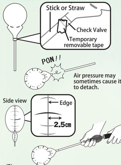
(2) Slowly insert air up to the size of the wrinkles in the figure, making sure that the stick doesn't detach from the balloon.
